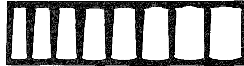
Fig. 5 Timewise evolution of the frozen layer for transitional freezing. Series III data runs: \Delta T_i = 13.9^\circ\text{C} , \Delta T_o = 17.8^\circ\text{C} . Freezing times (left-to-right): 30, 60, 90, 120, 150, 180, 240, and 300 min
